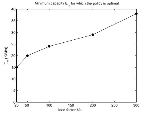
Fig. 9. Minimum required capacity  $E_m$  for which the policy is optimal, versus the demand load.
