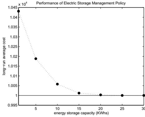
Fig. 5. Performance of the proposed energy storage control policy as a function of available storage capacity.
