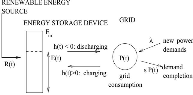
Fig. 3. Extension to the model, with a renewable source feeding the battery.
