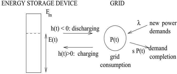
Fig. 1. Overview of system model with the energy storage device, the charging and discharging process, and the interaction with grid consumption.
