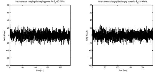
Fig. 8. Instantaneous charging / discharging power for  $E_m = 10$ KWhs and  $E_m = 24$ KWhs.
