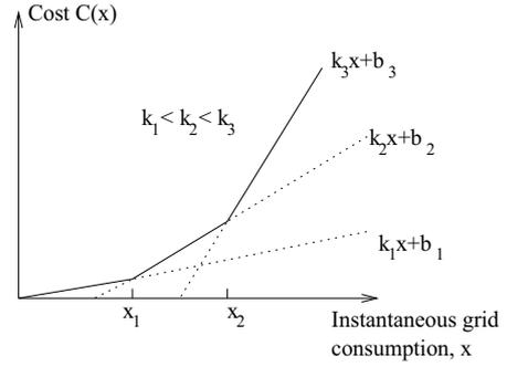
Fig. 2. The cost as a piece-wise linear convex function of the grid load.
