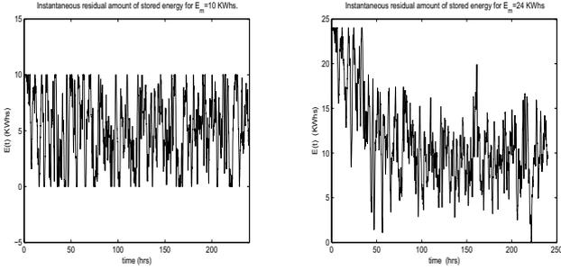
Fig. 6. Instantaneous residual amount of stored energy for  $E_m = 10$ KWhs and  $E_m = 24$ KWhs.
